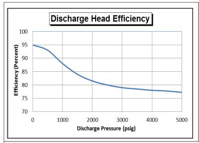
**NOTE:** With an increase in discharge pressure, the volumetric pumping efficiency of the pump head decreases as shown in the graph.
